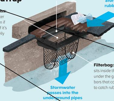
**Filterbag:** sits inside the drain, under the grating (the bars that cover the drain), to catch rubbish
